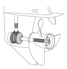
Yamaha's F70 provides outstanding hole shot and acceleration thanks in part to an advanced sensor that allows maximum safe ignition timing and a gearcase featuring a high 2.33:1 gear ratio, with specially hardened pinion, forward, and reverse gears for increased durability.
