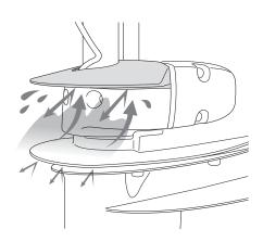
Yamaha's large anti-splash plate, standard on F70 models, helps keep water from splashing up between the leading edge of the outboard and the boat, resulting in a much dryer ride. Located on the front of the lower mid-section just above the lower unit, it excels in applications where the outboard is normally run deep in the water, such as pontoon boats.
