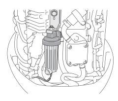
All new F70 outboards feature a large, on-engine water separating fuel filter with a water sensor. Used in conjunction with Yamaha's optional boat-mounted 10-Micron Water Separating Fuel Filter, it helps separate water and contaminants from the fuel before they can reach the outboard's other filters and fuel injectors.
