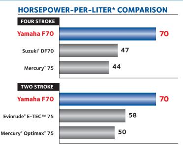
An advanced powerhead design features a single overhead camshaft (SOHC), yet with four valves per cylinder, for maximum power and efficiency. Total intake valve area is increased 17%, while the pistons and valves are up to 10% lighter (when compared to our T60 model), giving it substantially more horsepower-per-liter of engine displacement than competitive outboards, both four stroke and two stroke direct-injected.
