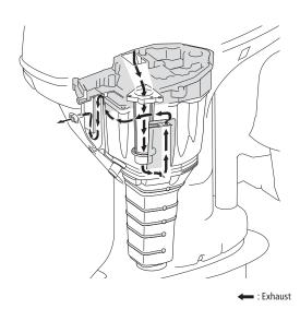
Engine exhaust is routed through a maze before exiting above the waterline through the idle exhaust relief outlet for unbelievably smooth and quiet operation.
