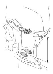
Yamaha's F70 four stroke outboard utilizes a Long Span Mounting System, which uses large specially-constructed rubber engine mounts placed as far apart vertically and horizontally as practically possible. Smooth and quiet operation, yet with strength and durability, is the result.
