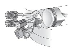
Four individual compact electronic fuel injectors deliver the exact amount of fuel needed for optimum performance and economy. Controlled by the Engine Control Module via input from an array of on-engine sensors, their location just above the intake valves enhances fuel atomization, resulting in more efficient combustion.
