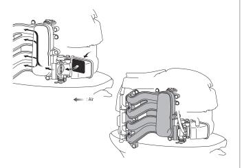
All air entering the engine block of Yamaha's new F70 four stroke is routed through a single throttle valve, to ensure density and power.
