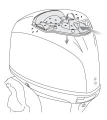
The new F70 features a new outer cowling design with an intake air drain system, to easily and efficiently drain away any water that enters the cowling during normal engine operation. Incoming air is routed through a labyrinth of passages that help trap and drain water before it enters the engine's intake, for maximum reliability.
