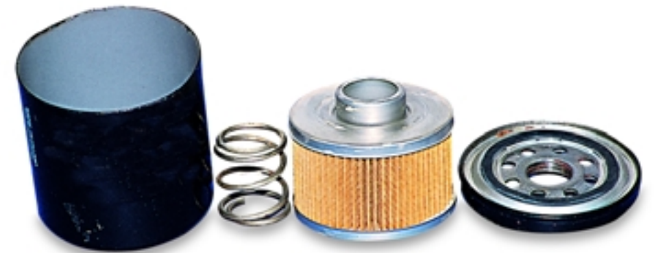
■ The basic components of a spin-on fuel filter help protect your engine from contaminants. The gray inside the canister is epoxy coating for rust resistance.
