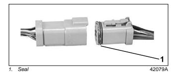
Connect outboard main wire harness to boat wire harness. Secure connectors in brackets.
