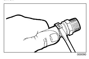
Method 3: Use Oetiker pincers (pliers) to grip clamp. Pull clamp off of connection and discard.
