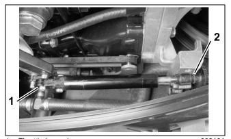
Throttle lever pin Trunnion nut
