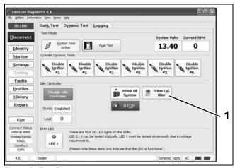
**Dynamic Test Screen**1. Prime Cylinder Oiler button
