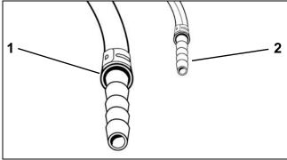
1. Fuel supply hose and fuel fitting - 3/8 in. (9 mm)
