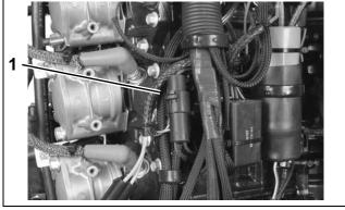
60° V4–V6 Models1. Accessory battery charge connector
