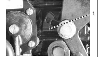
Throttle lever stop - 2 Cylinder models
