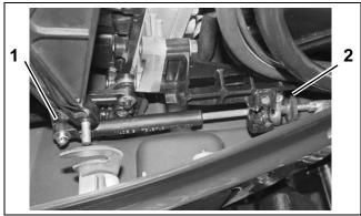
1. Shift cable retainer clip and washer
