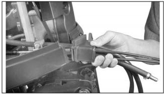
When grommet is in place and all cables have been installed, tighten a tie strap around the outside of the grommet to form a watertight seal around the cables.
