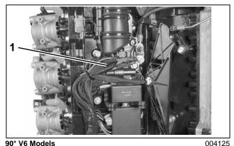
90° V6 Models1. Accessory battery charge connector
