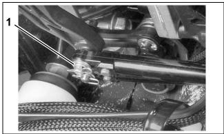
1. Throttle cable retainer clip and washer
