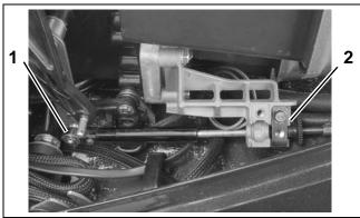
1. Shift cable retainer clip and washer
