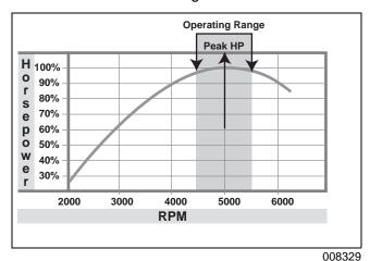
**NOTICE** If the propeller blades have too much pitch, the engine will operate below its normal range at full throttle. Power will be lost, and powerhead damage could occur. If the propeller blades have too little pitch, the engine will operate above its normal range and
