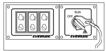
ICON style multiple start switches with master power/emergency stop switch
