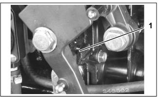
Throttle lever stop - 3 Cylinder models
