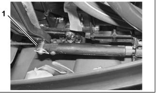
1. Throttle cable retainer clip and washer
