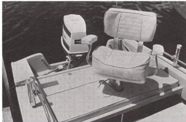
Stern Deck Assembly: Required on 17-foot Newports, Montauks and Stripers if Aft Pedestal Seat or Ski Pylon is to be installed. Solidly built and securely fastened. Stern Deck Cushion also available.
