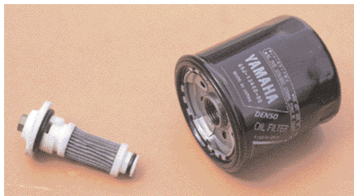
■ Most four-stroke outboards use canister-style oil filters that need to be replaced after 100 hours of use. Smaller engines utilize oil screens that require periodic cleaning.
